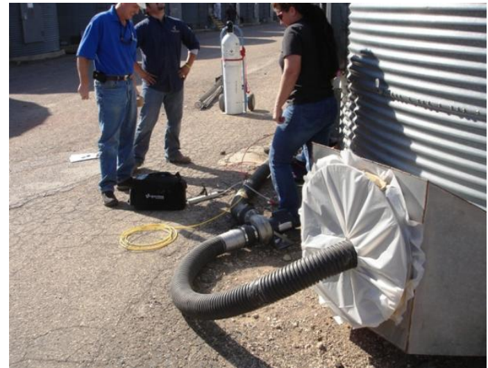
J-fan system with yellow introduction hose installed in front of fan
